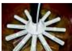
COLECTOR DE BRAZOS COLLECTOR WITH LATERALS
