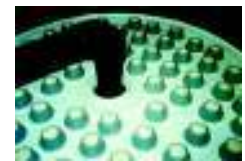
PLACA CON CREPINAS WITH NOZZLES PLACE
