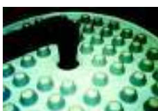
COLECTOR DE PLACA COLLECTOR PLATE WITH NOZZLES
